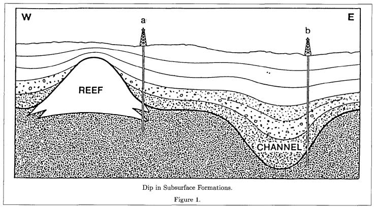
measures the conductivity of rock in a number of directions around the borehole. Variations in conductivity can be correlated and combined with measurements of the inclination and orientation of the tool to estimate the magnitude and azimuth of the dip or tilt of various formation layers penetrated by the borehole (Figure 1).
