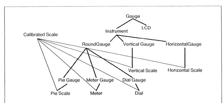
In this arrangement, a CalibratedScale mixin is created for tick marks and labels. In this reorganization there is a CalibratedScale mixin which is added to uncalibrated classes to create tick marks. For example, VerticalScale is a subclass of VerticalGraph and uses the CalibratedScale mixin.
