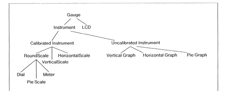
This lattice shows gauges partitioned into CalibratedInstrument and UncalibratedInstrument which exploits the observation that the best-looking uncalibrated instruments are also the space-filling ones. However, code is duplicated, for example, between HorizontalScale and HorizontalGraph.
