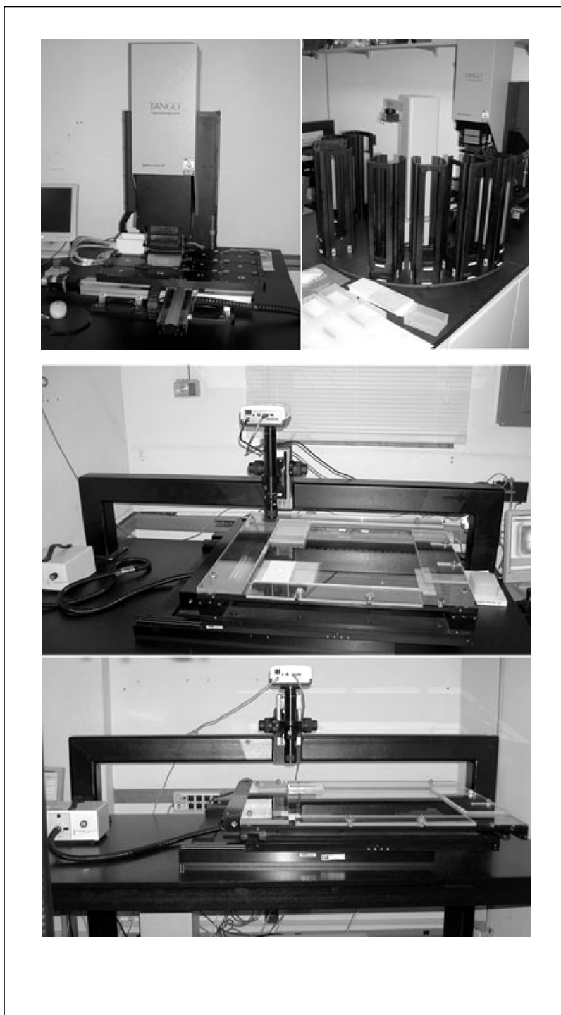
Figure 2. Crystallization Solution and Protein Pipetting Robots and XY Photography Stands.
